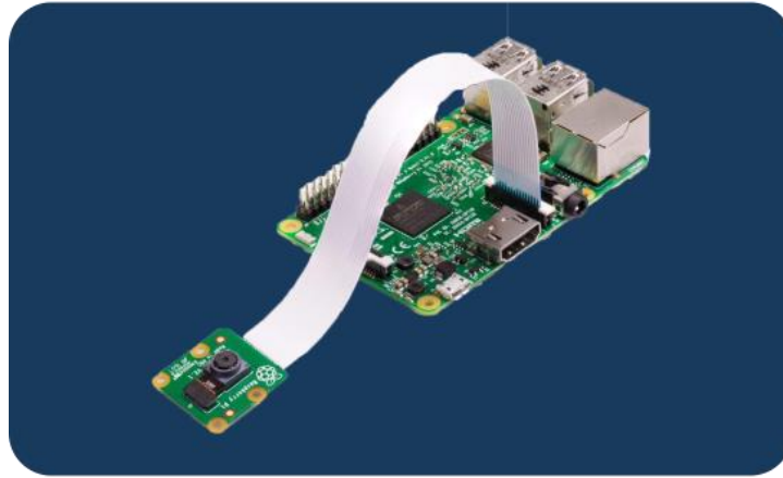
Figure 4: The body camera consisted of a Raspberry Pi computer with the Camera Module V2
