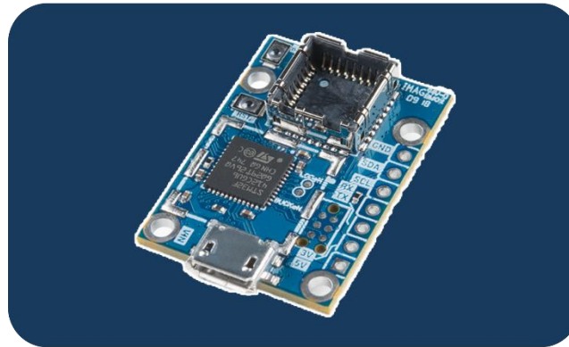
Figure 10: PureThermal 2 Lepton smartboard
