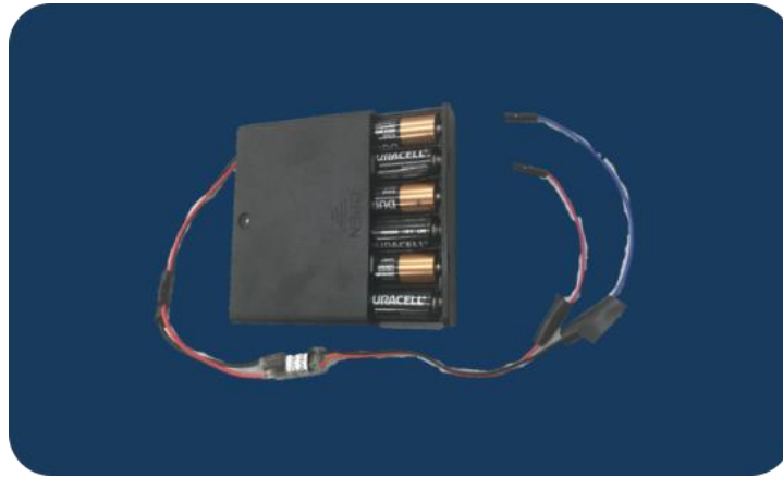
Figure 13: AA battery pack with UBEC volt dropper
