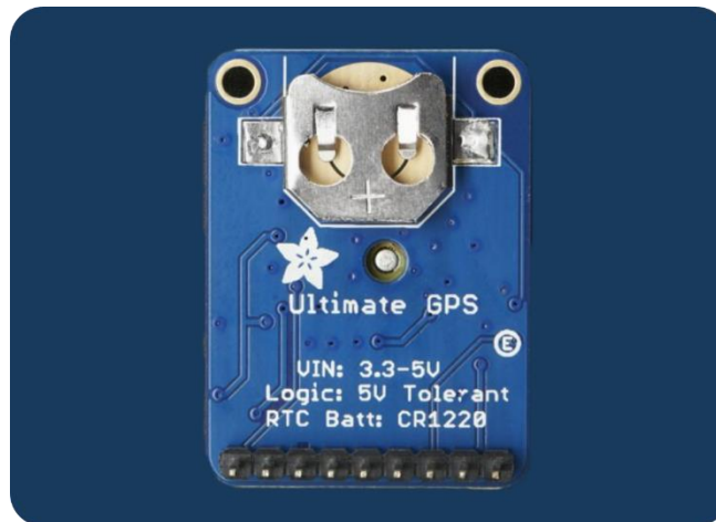
Figure 6: Optional pill battery emplacement for the GPS module
